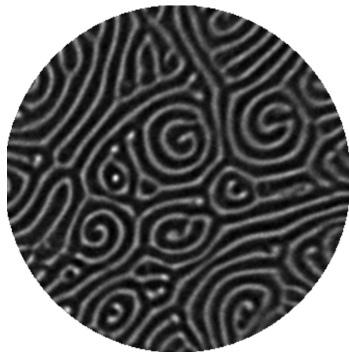
Figure 2: An image of the “prepared pattern” formed by Rayleigh-Bénard convection. A thin layer of fluid is heated from below and cooled from above. Dark regions indicate the hot upflows and bright regions indicate cold downflows. Adapted from H. Kurtuldu, K. Mischaikow, and M. Schatz, “Measuring the departures from the Boussinesq approximation in Rayleigh-Bénard convection experiments,” Journal of Fluid Mechanics , vol. 682, pp. 543–557, 2011.
